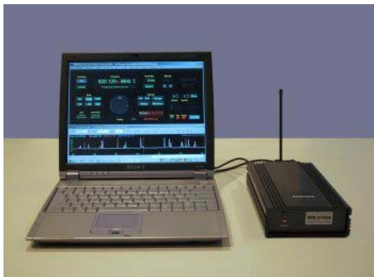
Figure 1 Computer-Controlled Radio And Laptop Computer Used To Perform EMI Measurements.
