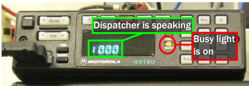
Figure 2 – Motorola W7 Control Head - Dispatcher Transmitting
