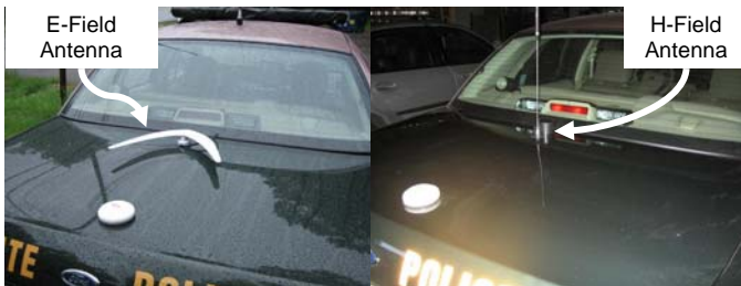
Figure 1. Electric and Magnetic Field Antennas Mounted on Police Vehicles. The H-Field Antenna Is Positioned Just in Front of the Vertical Whip.
